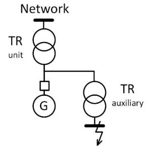
$$S_B = S_{atn} = 20 \text{ MVA}, U_B = 6 \text{ kV}$$
