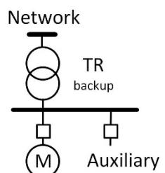
Motor:  $S_{nM} = 4 \text{ MVA}$ ,  $U_{nM} = 10 \text{ kV}$ , startup current:  $i_{startM} = I_{startM} / I_{nM} = 4 \text{ p.u.}$
